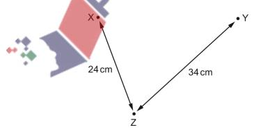
When the wave generators operate in phase, the amplitude of oscillation at Z is zero.
