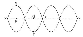
The solid curve shows the string at a position of maximum displacement. The dashed curve shows the other position of maximum displacement. The straight central dashed line shows the mean position of the string. Point S on the string is directly above point P. Point T on the string is directly below Q.
