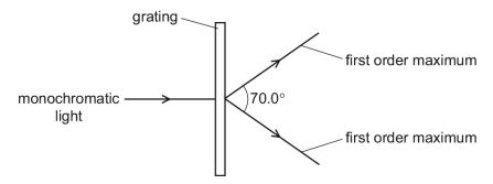
The spacing of the slits in the grating is  $1.00 \times 10^{-6}$  m. The angle between the first order diffraction maxima is  $70.0^{\circ}$ .
